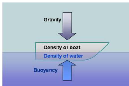
› When a boat is placed in water, it displaces an amount of water equal to the boat's weight – as long as the object is less dense than the water, it will float.
