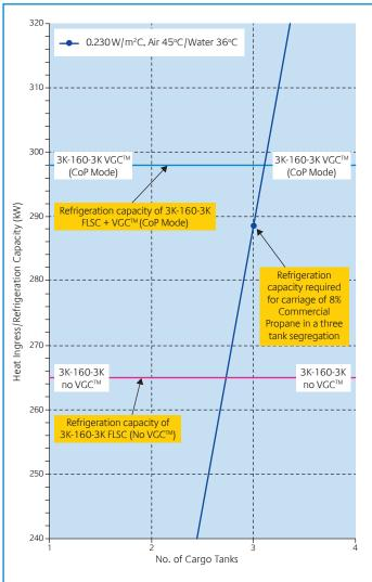
The refrigeration capacity required for fully refrigerated carriage of a 3 tank segregation of Commercial Propane
