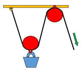
The amount of effort that is required to lift the object can be greatly reduced by adding two or more wheels together. As more pulleys are added, you increase your **mechanical advantage**. This means it becomes increasingly easier to lift the same load. The only difference is that you need a longer piece of rope/chain to lift the same load.
