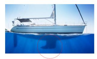
Keels carry ballast (gives the boat stability) by being made from a heavy material. The keel's broad, flat surface helps create sideways force by displacing water in the opposite direction that the boat is leaning. Although the keel is much smaller than the sails, the density of the water allow its force to be strong enough to stop the sailboat capsizing.
