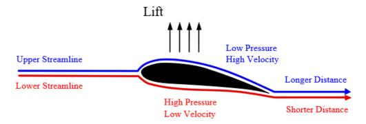
Now imagine a sail is a plane wing on its side, where lift is a sideways force instead of an upwards force. But because the wind typically hits the sail from an angle, this means the lift is both in a sideways and forward direction. So there needs to be a solution to stop the boat drifting sideways and to only move forward.
