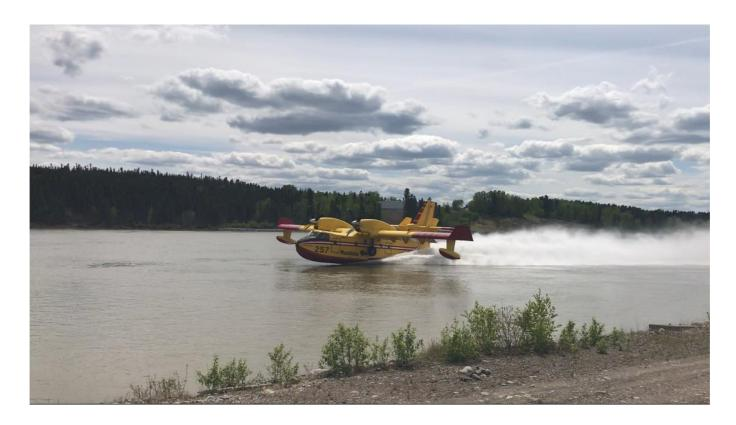
In our aerial firefighting operations, the centre of gravity of the Canadair waterbombers (pictured above) are constantly changing as they scoop up and release water over and over again. These aircraft can scoop up to 6,100 litres of water at a time so our pilots need to be highly aware of the change in centre of gravity so that they can keep the aircraft level and counteract the gravitational forces.
